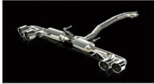
Slip-On Line+Tail pipe set
